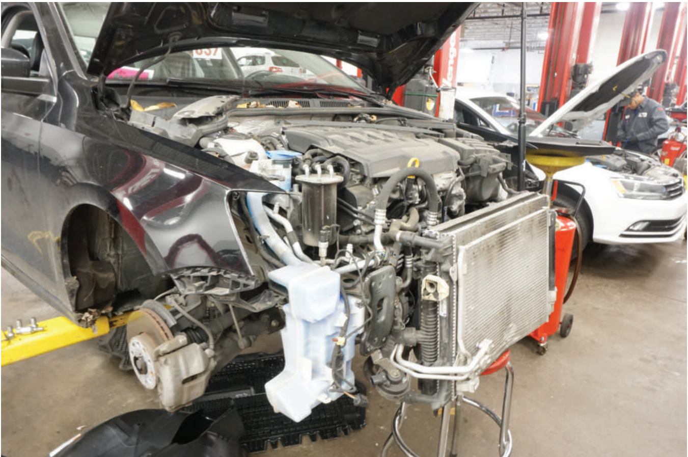
FIGURE 1-13 A service technician troubleshoots problems, performs all necessary diagnostic tests, and competently repairs or replaces faulty components.
