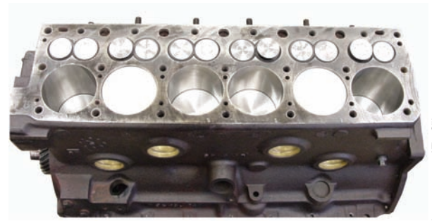
FIGURE B A flathead Studebaker block with the head removed.
