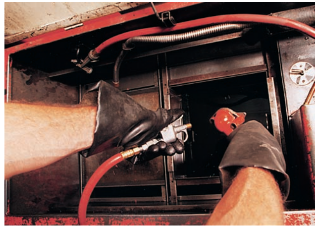
FIGURE 2.7 When drying parts with compressed air, blow solvent back into the solvent tank.
