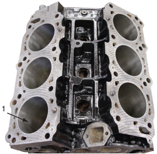
FIGURE 1.35 The number 1 cylinder is the closest to the front of the engine on almost all V-type engines.
