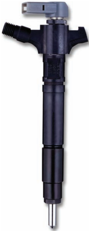
FIGURE 1.40 A special fuel injector designed to close against high pressure.
